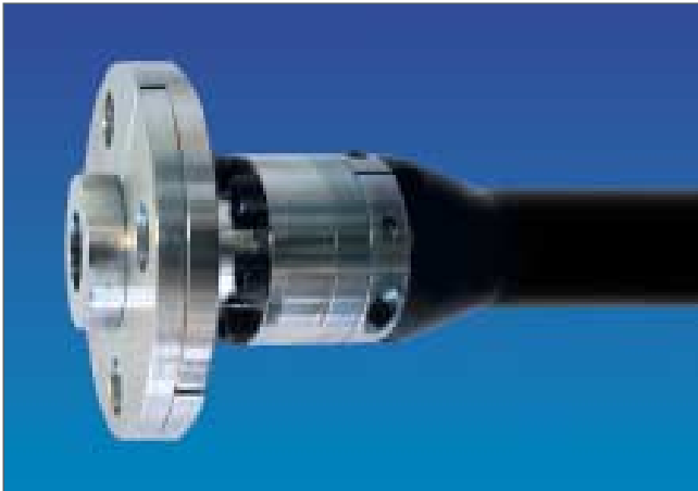
Fig.1: Installation of the FLEXWELL LPG connecting joints is made without the need for welding. A compression type fitting, using a graphite packing makes a perfect seal between the connector and the primary pipe, no specialised tools are needed for assembling this. The connecting joints are available with NPT pipe threaded ends or alternatively with a collar and split flanges for use with a standard flat gasket seal.
